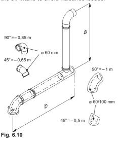
60 mm elbows and extensions can be added to the vertical section.
